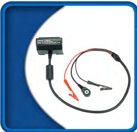
The **Smart Cable** features 4-wire battery cables with alligator clips to provide an easy connection to **larger batteries**. Ideal for batteries with exposed tabs or special terminals. The insulated alligator clips are connected to your Cadex analyzer by banana plugs. A magnetized temperature sensor is included to monitor the battery temperature.
